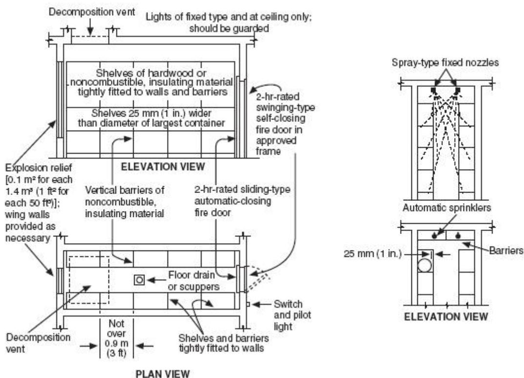
**FIGURE A.6.3 Standard Film Vault (for Other Than Extended Term Storage Film).**
