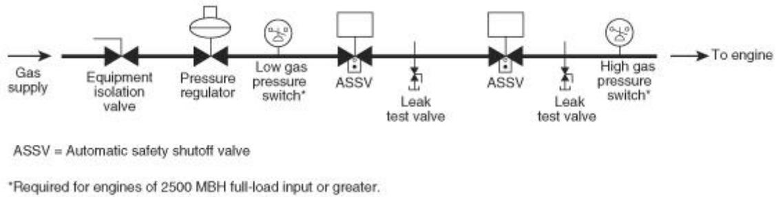
**FIGURE A.5.2 Typical Piping Arrangement of a Gas Train.**
