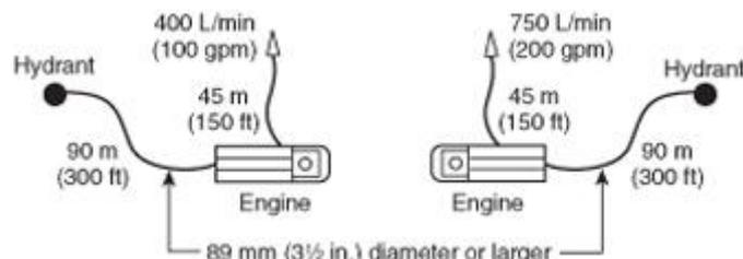
**FIGURE B.1.3 Forward Lays Using Two Engines.**
