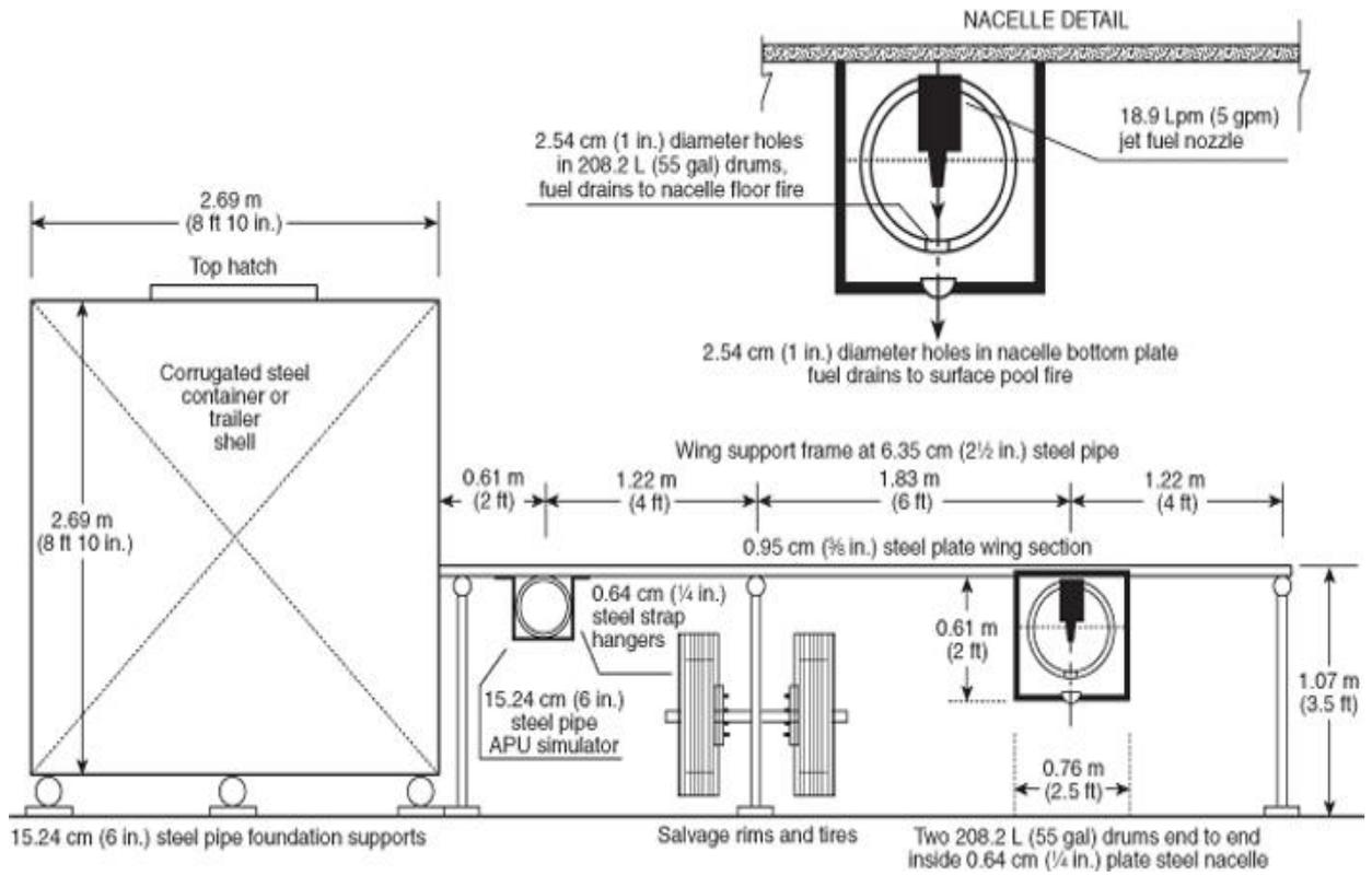
**FIGURE B.2(b) Aircraft Fire Suppression and Rescue Live Fire Training Mock-Up (front view).**
