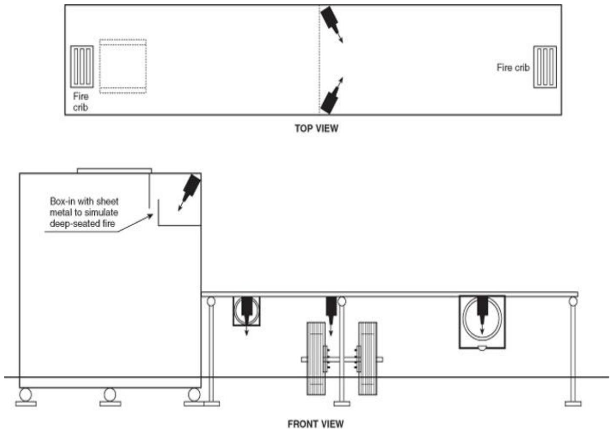
**FIGURE B.2(g) Aircraft Fire Suppression and Rescue Live Fire Training Mock-Up [liquid propane or atomized jet fuel nozzle locations (no scale)].**
