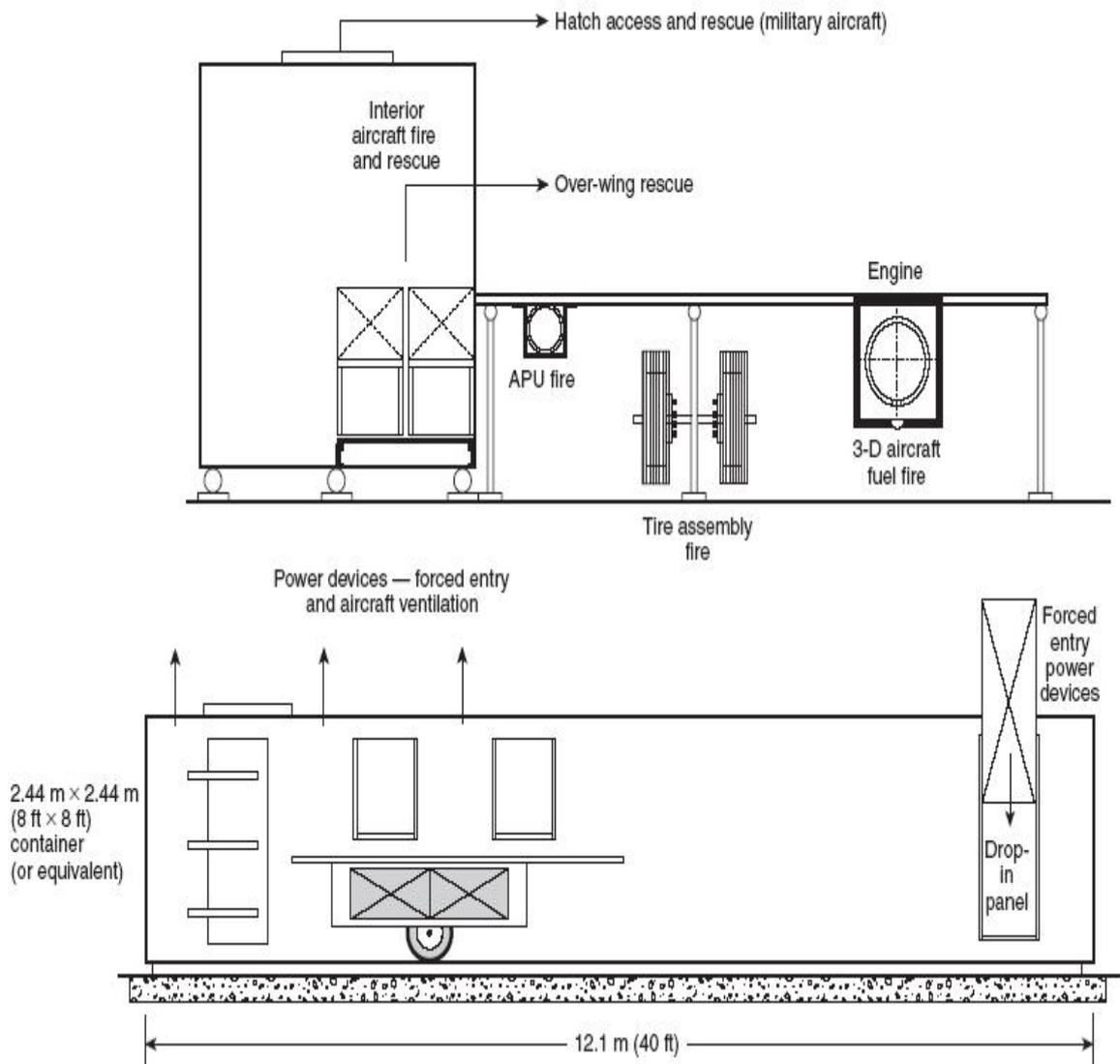
**FIGURE B.2(a) Aircraft Fire Suppression and Rescue Live Fire Training Mock-Up.**
