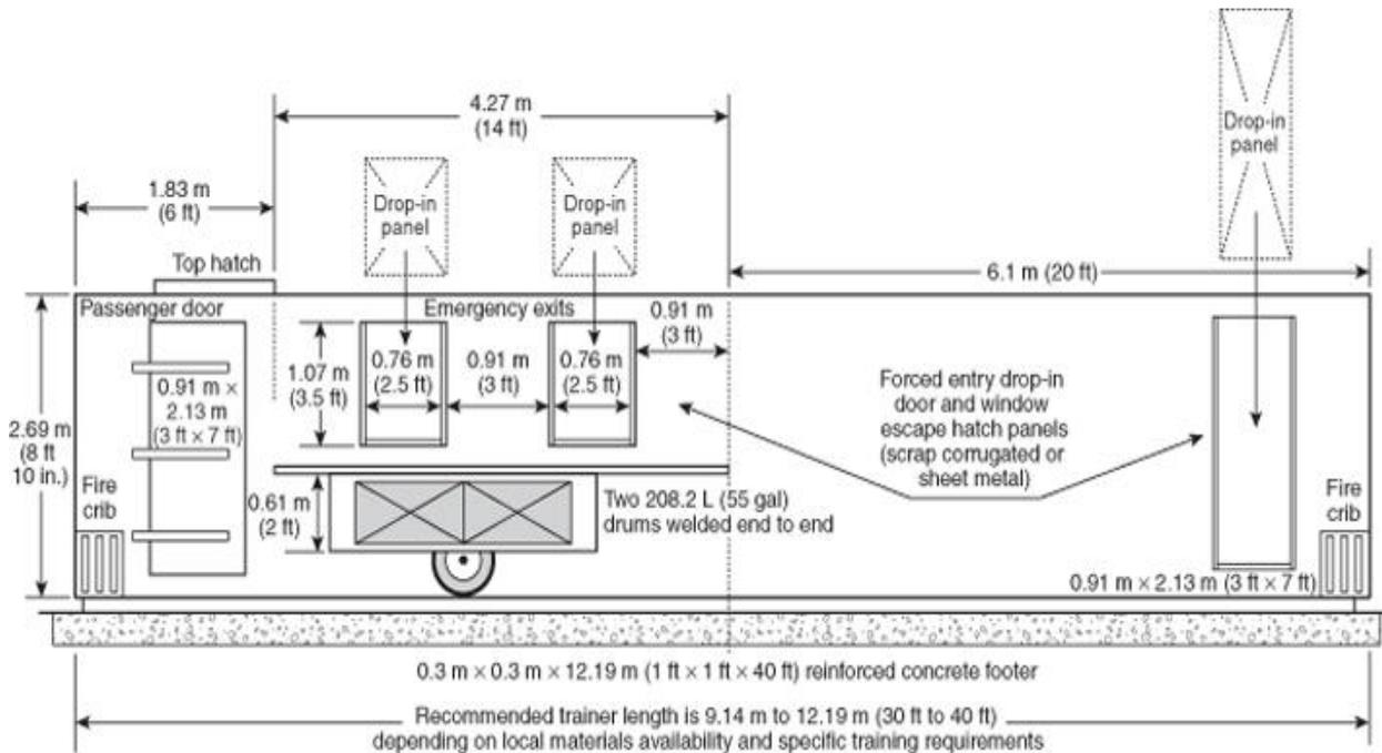
**FIGURE B.2(d) Aircraft Fire Suppression and Rescue Live Fire Training Mock-Up (over-wing egress side view).**
