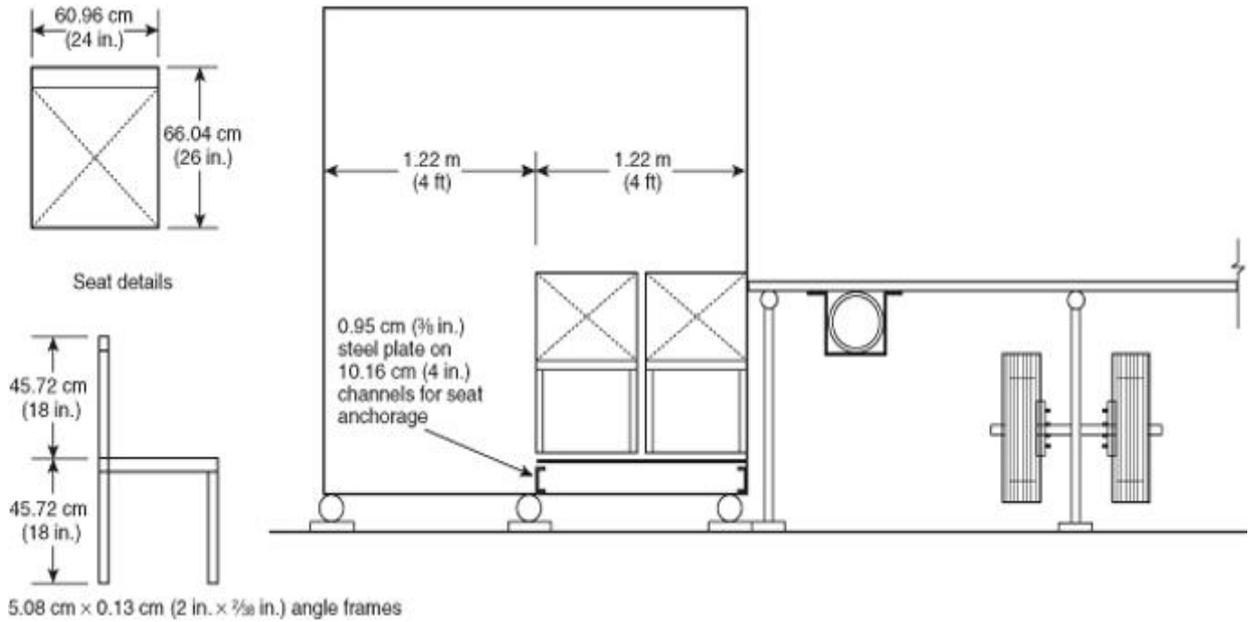
**FIGURE B.2(f) Aircraft Fire Suppression and Rescue Live Fire Training Mock-Up (interior seating arrangement).**
