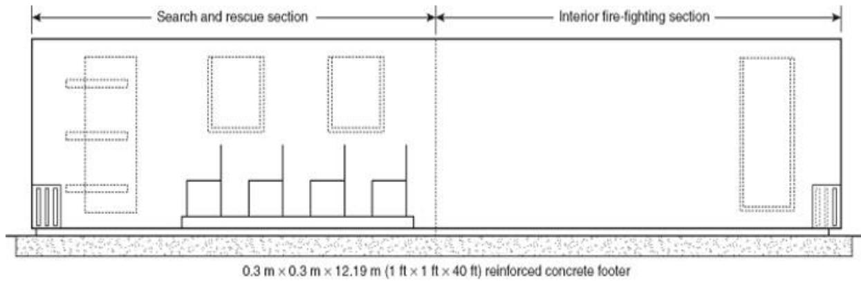
**FIGURE B.2(e) Aircraft Fire Suppression and Rescue Live Fire Training Mock-Up (interior aircraft seat arrangement).**
