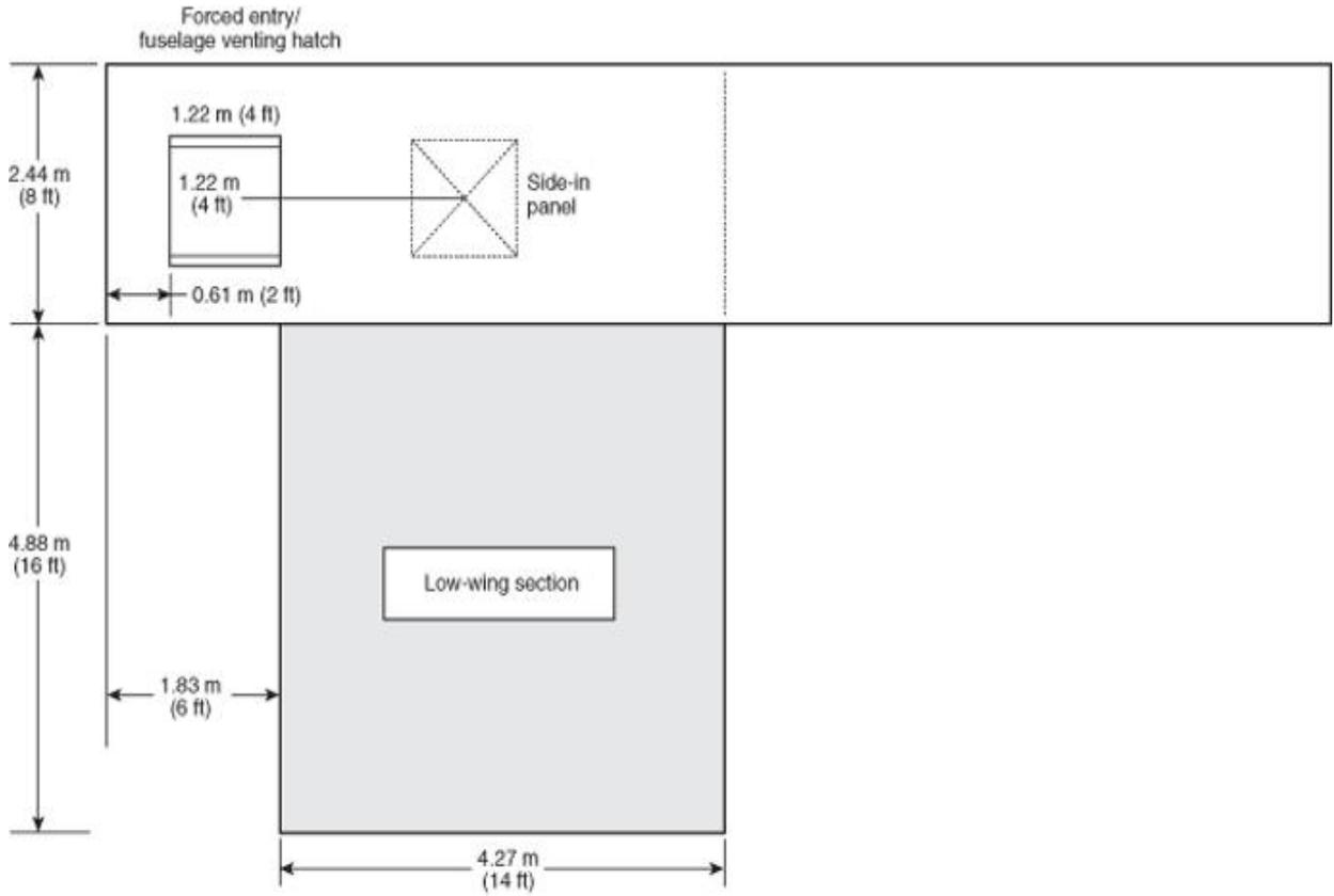
**FIGURE B.2(c) Aircraft Fire Suppression and Rescue Live Fire Training Mock-Up (top view).**
