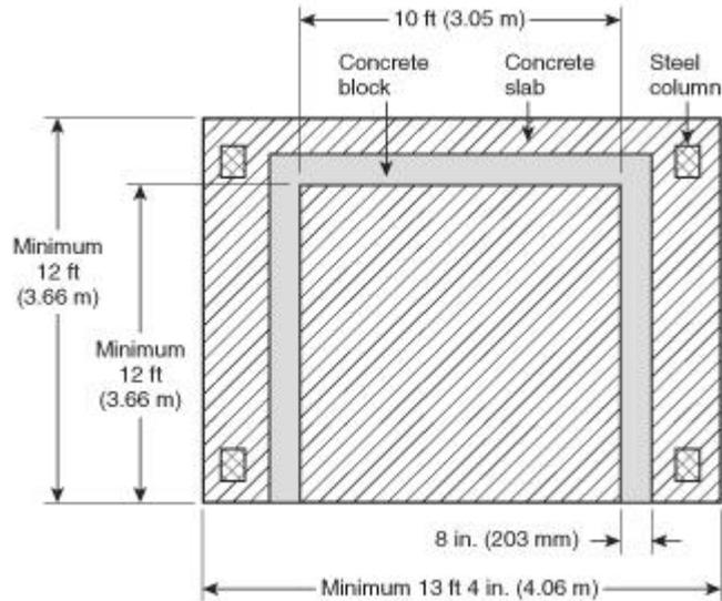
**FIGURE A.4.2.3(a) Front View of Test Apparatus (not to scale).**
