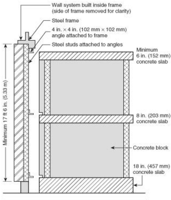
**FIGURE 5.2(c) Side View of Test Specimen in Movable Test Frame (not to scale).**
