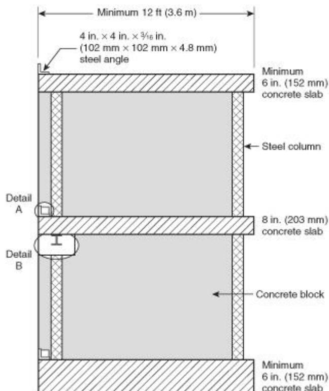
**FIGURE A.4.2.3(b) Plan View of Test Apparatus — Both Floors (not to scale).**
