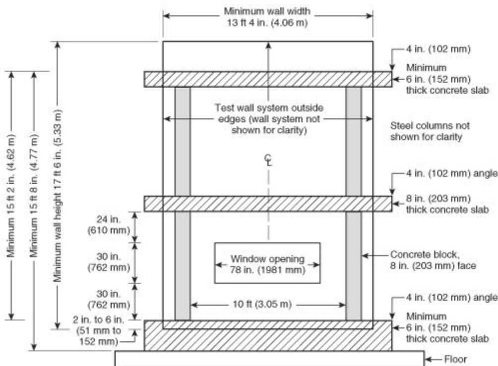
**FIGURE 5.2(a) Front View of Test Specimen Built in Place on Test Apparatus (not to scale).**
