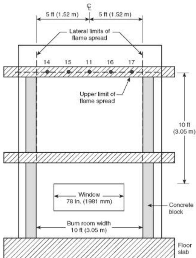
**FIGURE 10.2.1.2 Limits of Flame Propagation (not to scale).**
